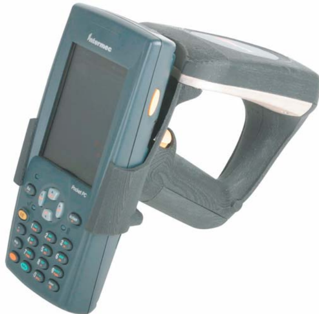
Figure 11. Intermec 750 with integrated AVI reader and pistol grip
